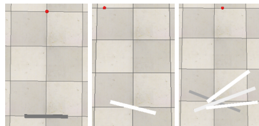
Fig. 3. For data collection, obstacles were systematically placed with varying orientation and height (left, middle), with different goal locations (shown with red dot). Data was also collected by randomly placing multiple obstacles in a similar fashion (right).
